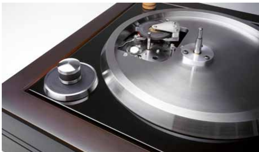
POWERFUL: The friction wheel on ruby bearings transmits the force from the 5 mm thick motor shaft onto the inside of the platter (removed here). The resulting torque is huge.
